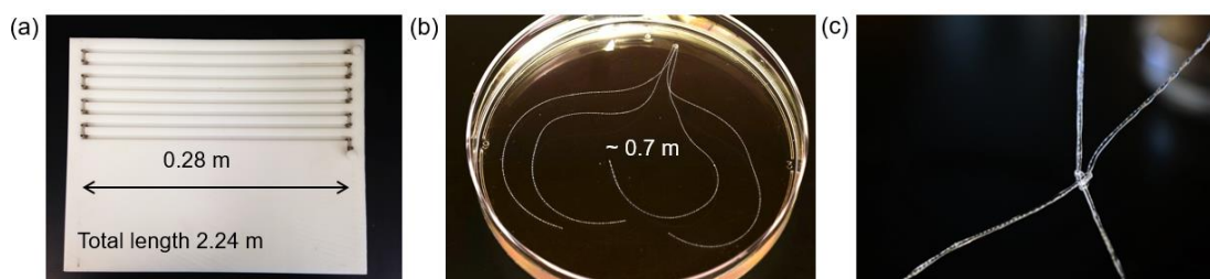
Figure S23. Scale-up of the device. a , Trough capable of fabricating a device of \sim 2.24 m. b , Device with 4 arms tied together with a total length of \sim 0.7 m. c , The knot region of the tied device.
